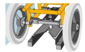
• In addition to securing wheelchairs using a four-point tiedown, wheelchairs can also be secured using a docking tiedown device. This method is primarily used in private vehicles since it requires the addition of adaptor hardware to the wheelchair frame that will engage with the docking tiedown device in the vehicle. Docking securement devices allow the wheelchair rider to secure and release the wheelchair without assistance.
