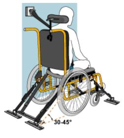
It is important to use a complete WTORS to secure the wheelchair and provide the wheelchair occupant with a properly designed and tested seatbelt system.
